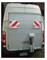
These tail lifts all function hydraulically and are equipped with an automatic tilting system.
